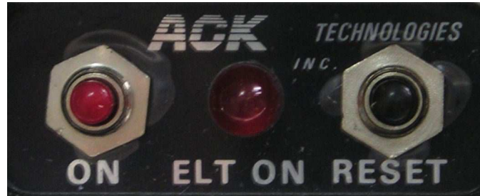
Figure 7.22: ELT Remote Control
