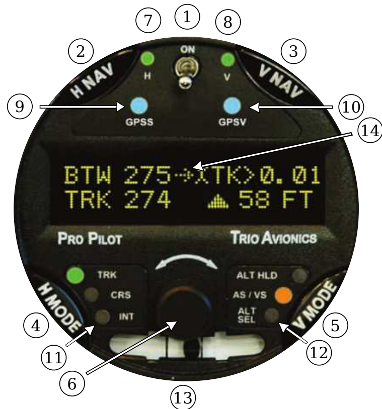
Figure 7.20: Trio Pro Pilot Autopilot
