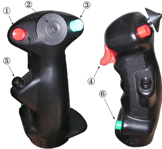
Figure 7.4: Stick Grip Switches
