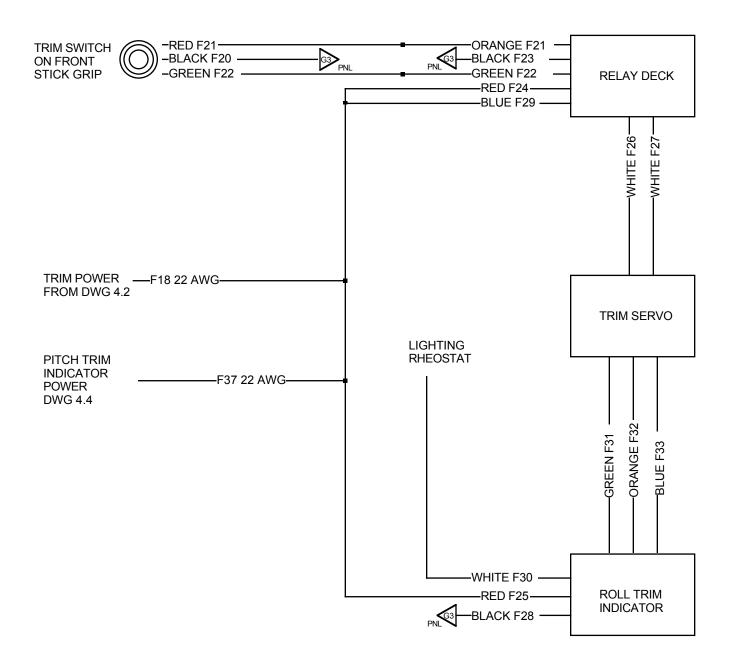
NOTES: 1. Wires with no size indicated are permanently attached to components supplied with trim system.
